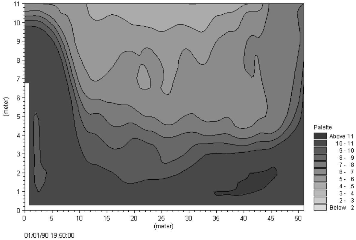
Figure 9: Salinity [%] in Section C-C at t = 19:55 (fully developed flood)
