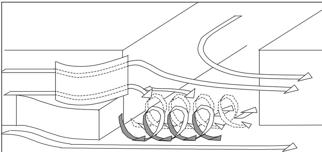
**Figure 3: Schematic Flow Pattern in Entrance during Flood with CDW present (VAN LEEUWEN and HOF LAND, 1999).**
