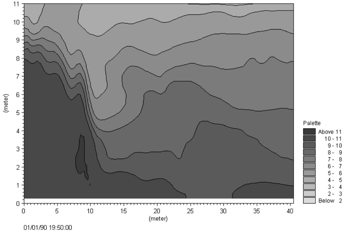
Figure 13: Salinity [%] in Section E-E at t = 19:55 (fully developed flood)
