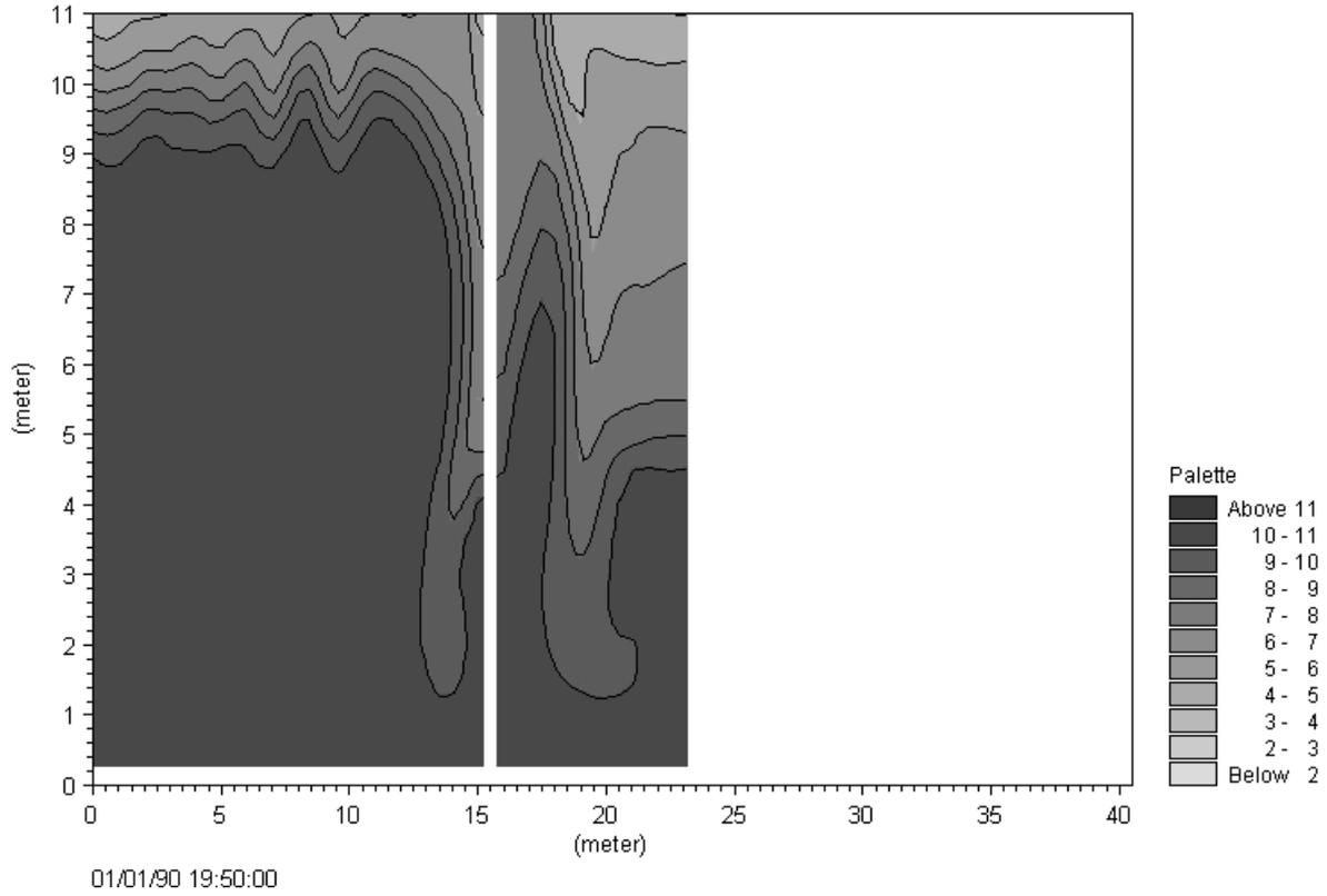
Figure 11: Salinity [%] in Section D-D at t = 19:55 (fully developed flood)
