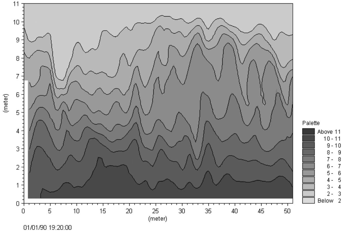
Figure 7: Salinity [%] in Section C-C at t = 19:20 (start of rising tide)
