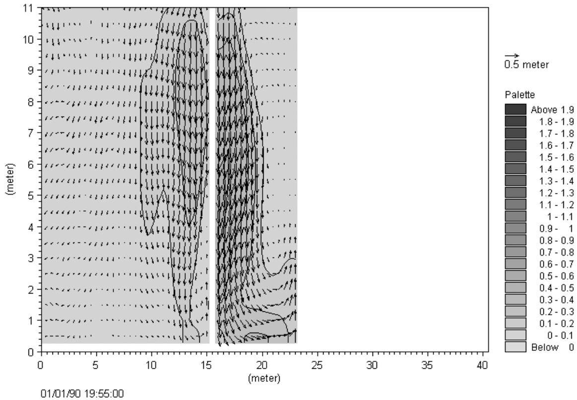
Figure 12: Flow Velocities [m/s] in Section D-D at 19:55 (fully developed flood)
