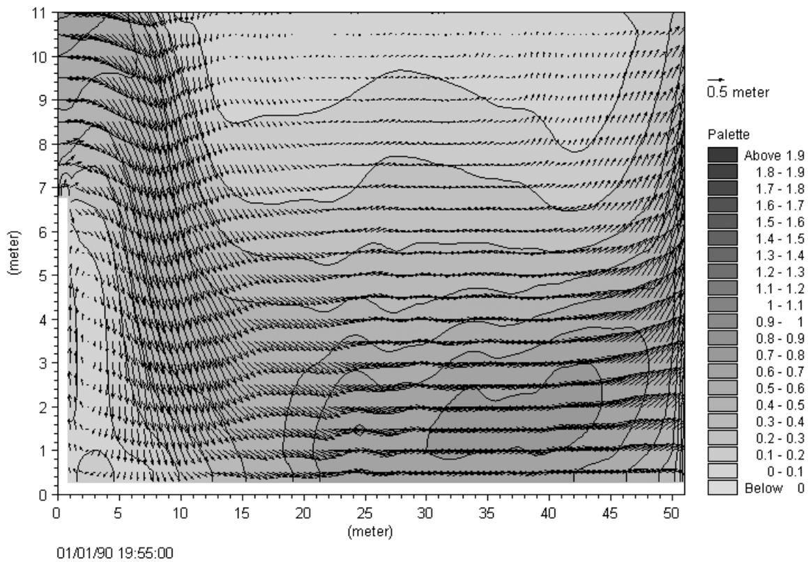
Figure 10: Flow Velocities [m/s] in Section C-C at 19:55 (fully developed flood)
