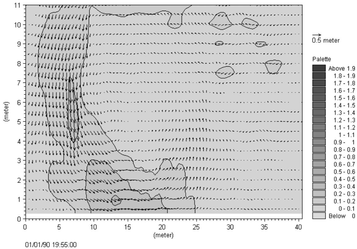
Figure 14: Flow Velocities [m/s] in Section E-E at 19:55 (fully developed flood)
