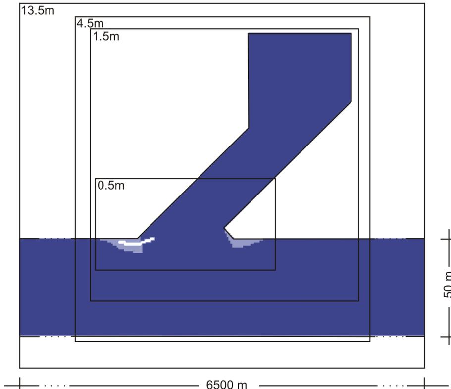
Figure 4: Grid Resolution of different Model Areas
