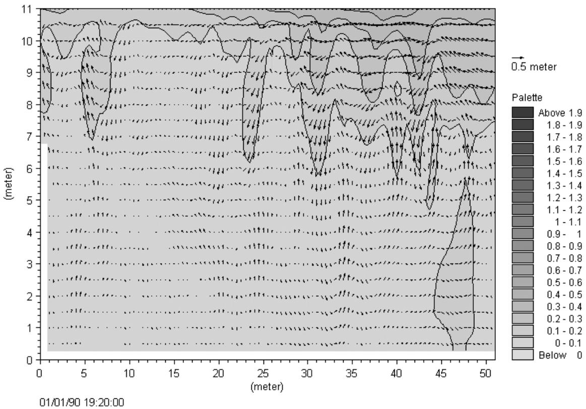
Figure 8: Flow Velocities [m/s] in Section C-C at 19:20 (start of rising tide)
