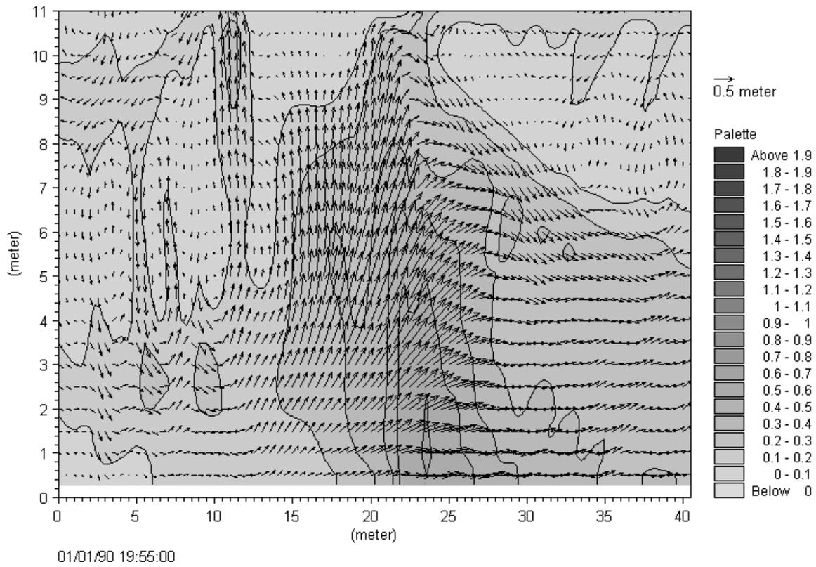
Figure 16: Flow Velocities [m/s] in Section F-F at 19:55 (fully developed flood)
