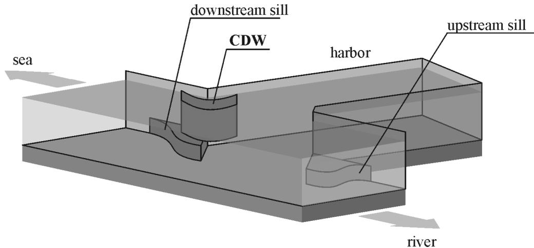
**Figure 1: Current Deflecting Wall downstream a Tidal Harbour Entrance**
