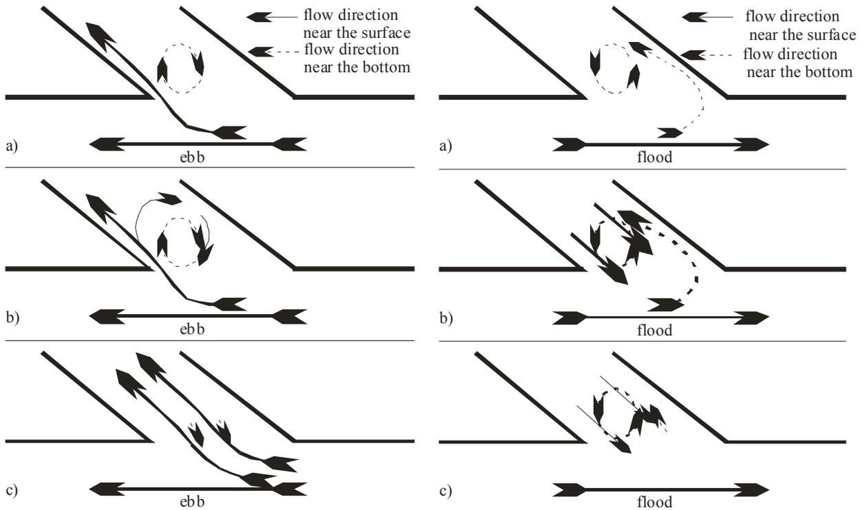
**Figure 2: Flow Pattern in the Harbour Entrances during Ebb (left) and Flood (right): (a) Beginning of Ebb/Flood, (b) During Ebb/Flood and (c) End of Ebb/Flood (FRANZIUS-INSTITUT, 2003)**
