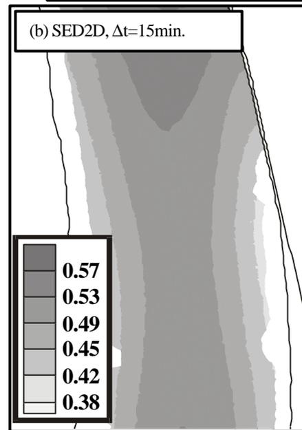
Figure 9: Sedimentation [m/year] in Neustadt Harbour (Entrance) for identical Boundary Conditions during Calibration Tests: (a) MIKE21,  $\Delta t=5\text{sec}$ . (b) SED2D,  $\Delta t=15\text{min}$ .
