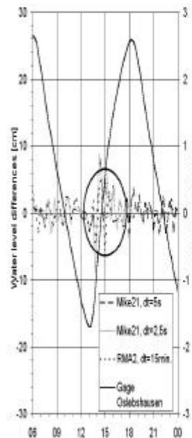
Figure 4: Water Levels/Differences at Gage Oslebshausen UW-km7.5 (17.03.1990 0000-17.03.1990 0000).
