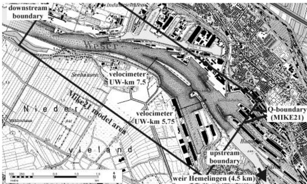
Figure 1: Model Area: FE-Mesh (RMA2/SED2D: combined triangular/quadratic mesh, element size 25-3200m<sup>2</sup>, 16078 elements) and FD-Mesh (MIKE21: starting point: 3482900,5884200; grid dimension: nx=500, ny=1090; grid resolution: dx=dy=5m; rotation against north=305°).
