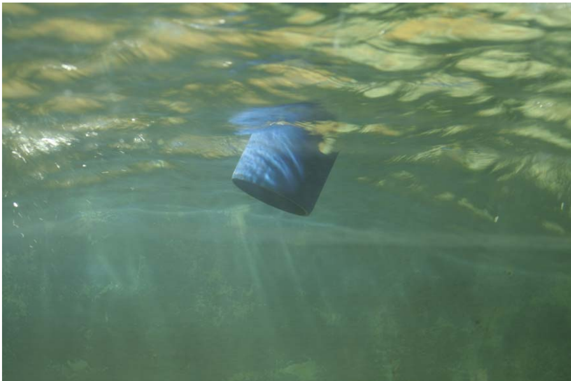
Figure 8: Orifice of “Wave Tube” Immersed by Passing Wave
