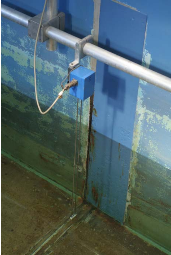
Figure 3: Resistance Type of Wave Gauge
