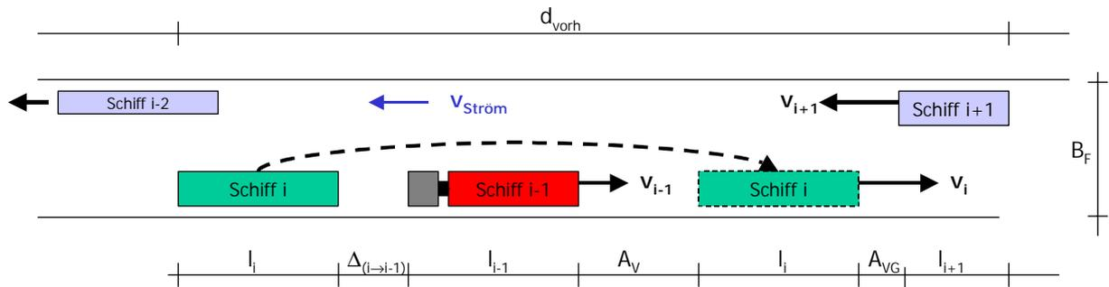
Fig. 4: Parameters used for Passing Simulation in WABIS Traffic Simulation Module
