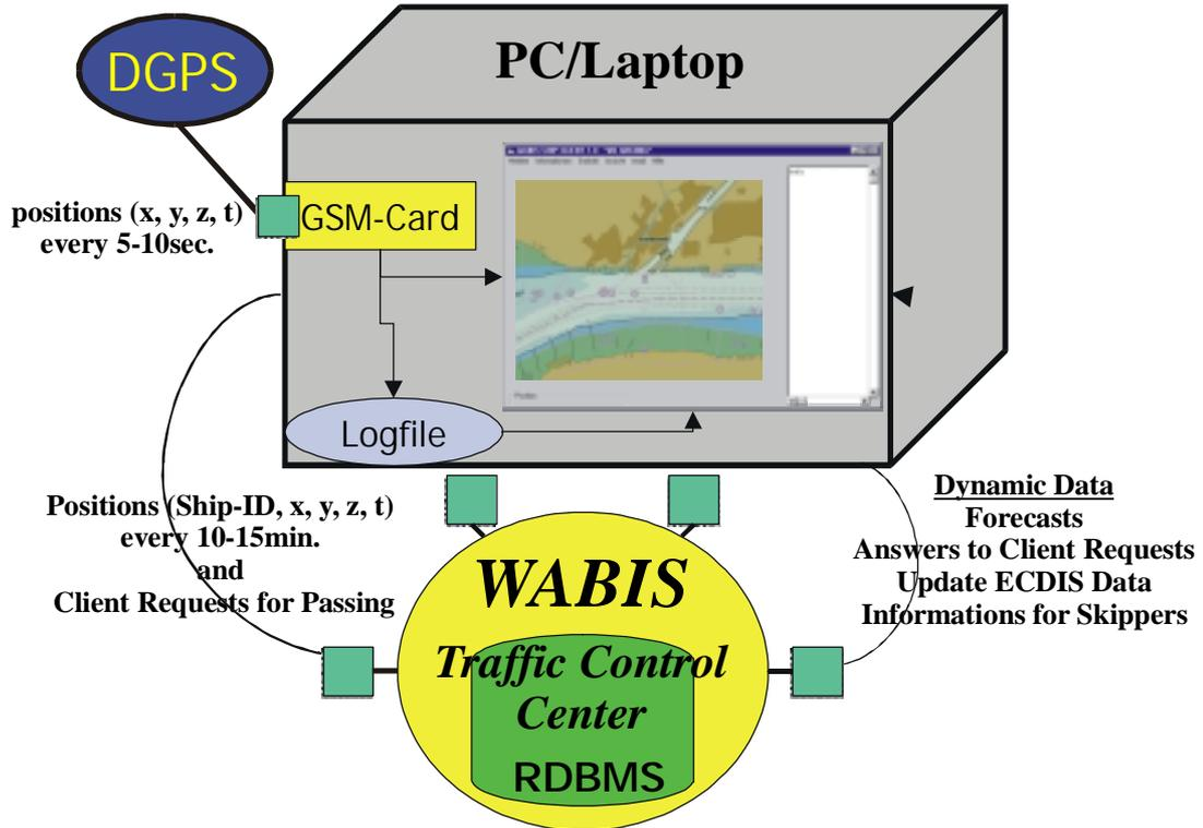
Fig. 2: On Board Communication GPS Transponder – WABIS Ship Client
