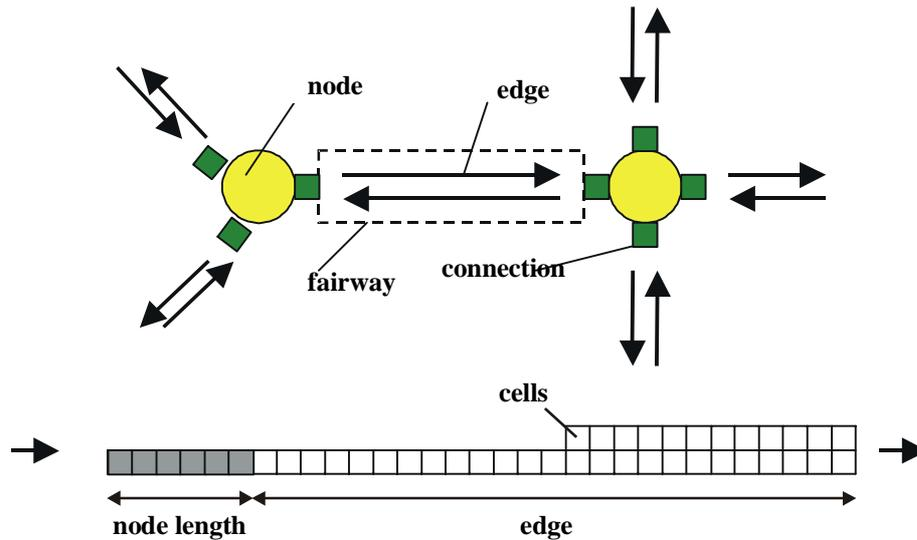
Fig. 3: Network Design with Edges/Nodes and Edge Splitting to model Vessel Traffic on Inland Waterways
