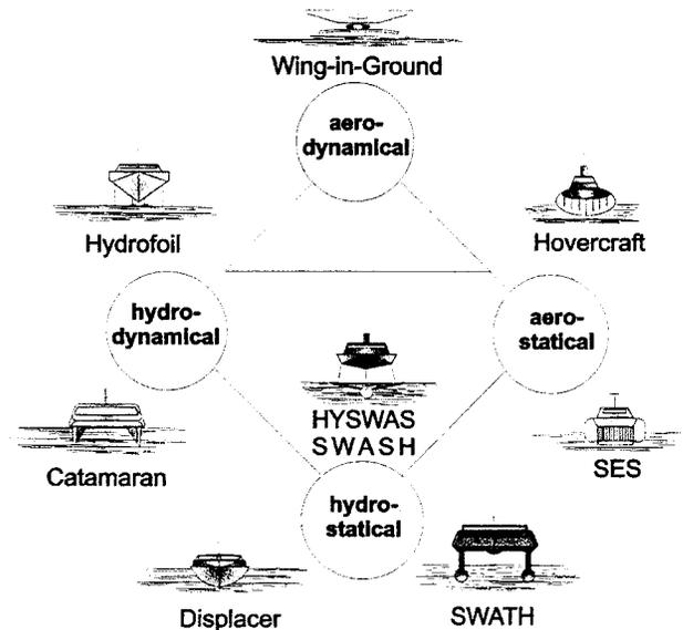
FIG. 5. Basic Types of High Speed Ships (Nitz and Muxfeld 1993)
