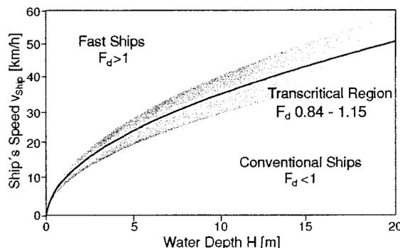
FIG. 1. Critical Speed in Depth Restricted Waters
