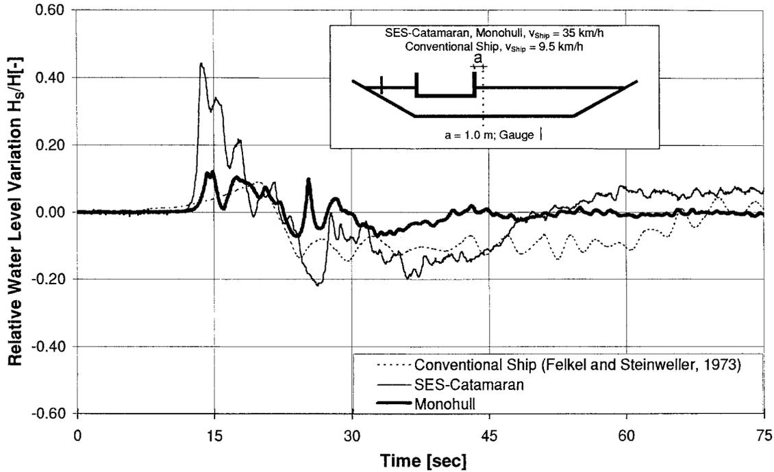
FIG. 6. Water-Level Variations for Different Ship Types and Ship Speed
