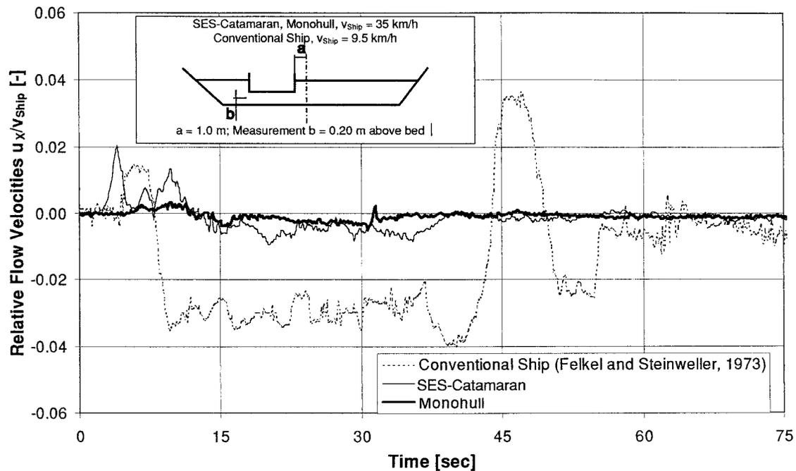
FIG. 7. Flow Velocities under Passing Ships at Fixed Location
