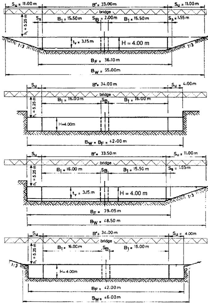
FIG. 4. Cross Sections of Canals in Germany
