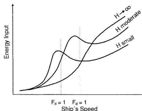
FIG. 2. Basic Relations between Ship Speed, Wave Resistance, and Energy Input (Schneekluth 1988)
