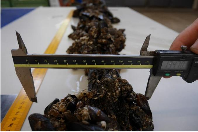
Figure 2: Blue mussel (*Mytilus edulis*) dropper line specimen 1 during preparation for drag testing.
