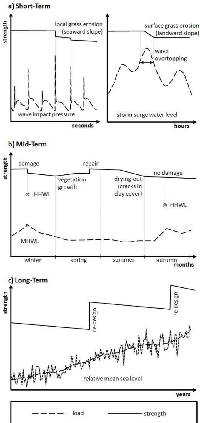
Figure 5. Loads and strength for different time scales: a) short-term, b) mid-term and c) long-term (Naulin et al., 2012)
