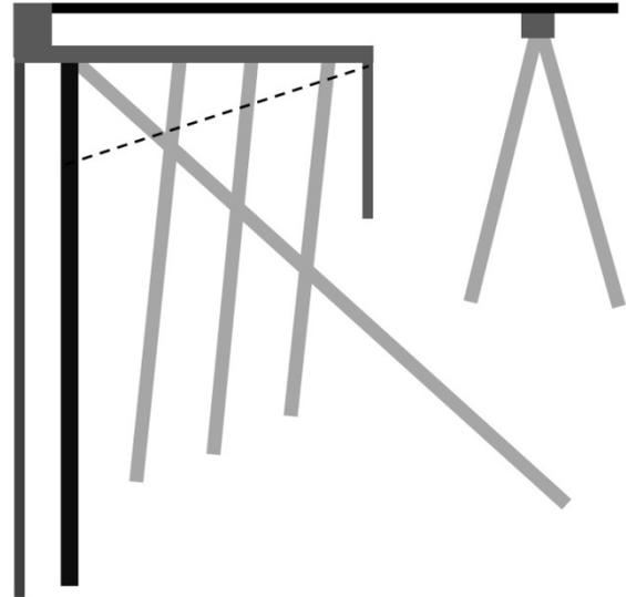
Figure 3. Sheet pile structure as a typical quay wall construction in German harbors (Principle sketch)
