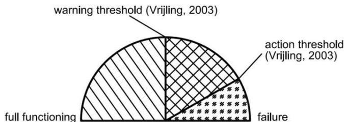
Figure 11. Scale for assessment of degradation (Principle sketch)
