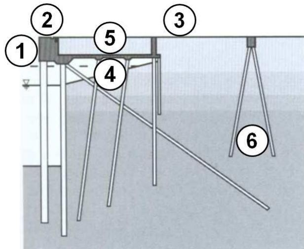
Figure 7. Different exposure classes for quay walls (Horstmann et al., 2012)
