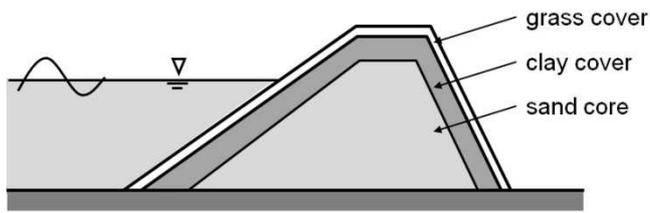
Figure 1. Typical dike cross-section at the German North Sea (Principle sketch)
