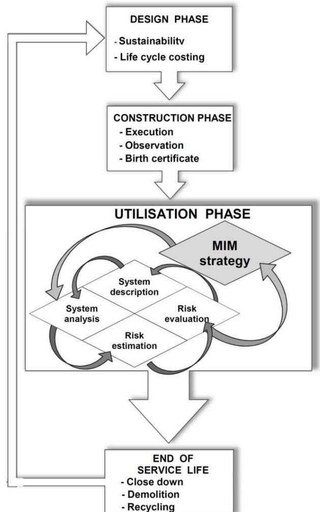
Figure 6. Life cycle phases including monitoring, inspection and maintenance (MIM) strategy (Horstmann et al., 2012)
