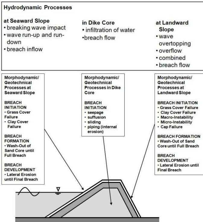
Figure 2. Overview of processes and failure mechanisms leading to dike breaching (Naulin et al., 2012)
