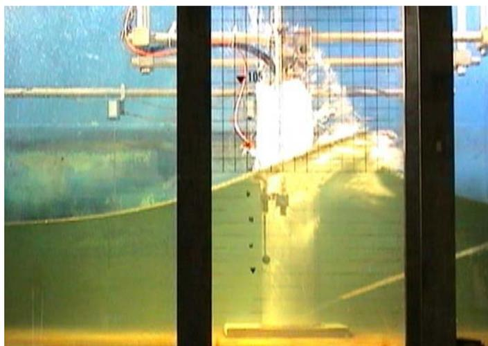
Figure 4. Breaking wave on cylinder
