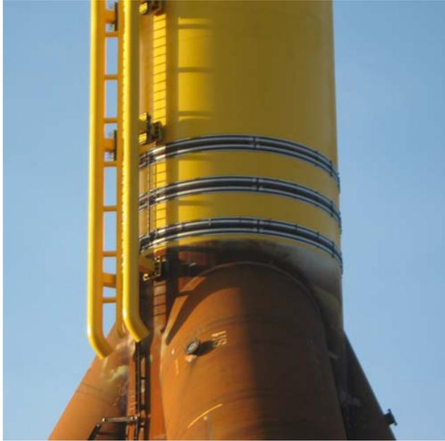
Figure 1. Tripod with 3 equipped belts
