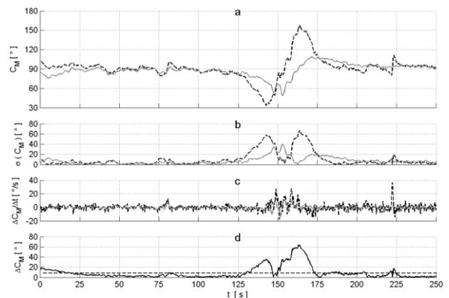
**Figure 1.** Comparison of internal and external magnetic compasses. a: Heading, b: Deviation from basic course, c: Change of heading, d: Absolute difference. In a-c internal compass is given in dashed black line, external compass is given in solid grey line
