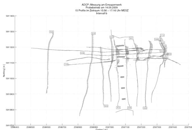
**Figure 6.** Overview of transects in the period of 15:54-17:16 MESZ at the river barrage 'Emssperrwerk' during trial operations on 14 September 2009. The northernmost secondary opening (NÖ1) and four southern secondary openings (NÖ2-5) are closed. Only main navigation opening (HSÖ) and inland navigation opening (BSÖ) remain fully open.
