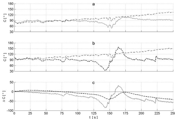
**Figure 2.** Comparison of magnetic compasses and rate of turn sensor. a: External magnetic compass and integrated rate of turn, b: Internal magnetic compass and integrated rate of turn, c: Absolute difference between magnetic compasses and integrated rate of turn. Internal magnetic compass in solid grey line, external magnetic compass in black dashed line and rate of turn information in dark grey dash-dotted line.
