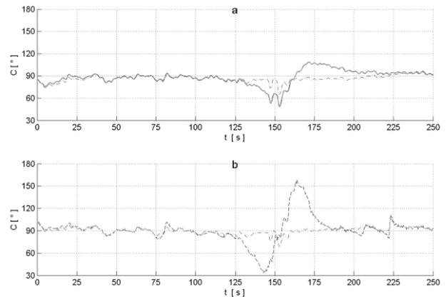
**Figure 3.** Heading from magnetic compasses corrected using rate of turn information from gyro sensor. a: External magnetic compass, b: Internal magnetic compass. Corrected heading is given in dash-dotted dark grey line.
