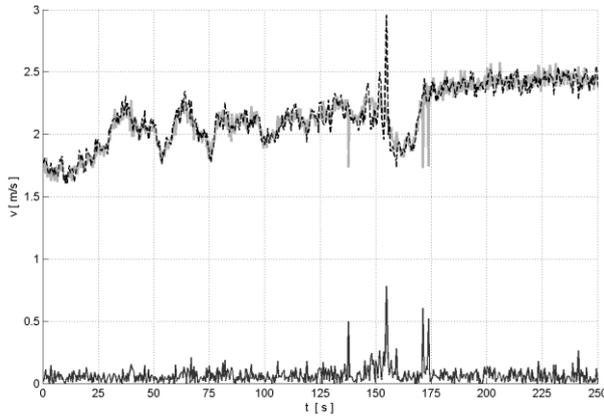
**Figure 4.** Comparison of instrument velocity obtained by GPS and bottom track. GPS velocity is given in solid grey line, bottom track velocity is given in dashed black line. Magnitude of difference is given in solid black line.
