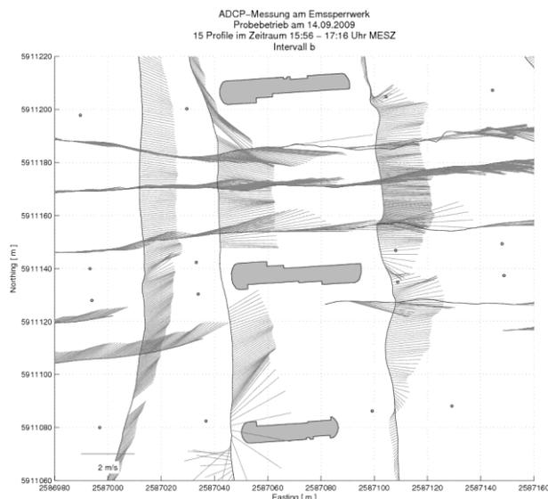
**Figure 7.** Close view of the flow field in main navigation opening (HSÖ) and inland navigation opening (BSÖ) during flood tide stream. Adjacent secondary openings are fully closed.
