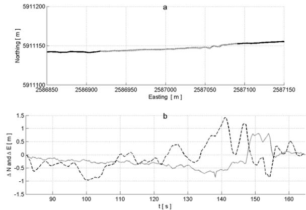
**Figure 5.** a: Dead reckoning reach after scaling and rotation. Original GPS track is given in solid black and dotted black line. Dead reckoning reach is given in solid gray line. b: Absolute error in Northing given in black dashed line and absolute error in Easting given in solid grey line.
