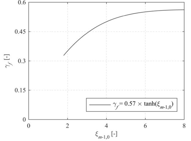
Figure 8. Reduction coefficient  $\gamma_f$  over Iribarren number.
