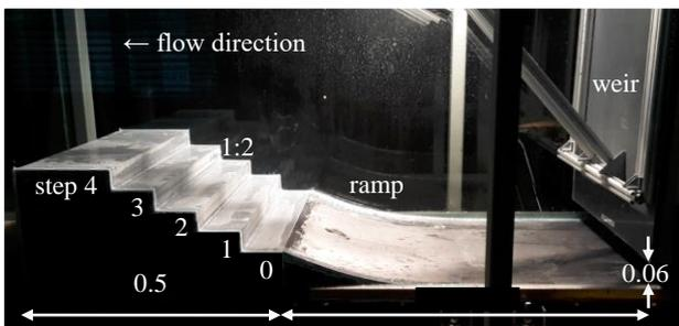
**Figure 4.** Set-up in the current flume, flow direction from right to left, measures in [m].
