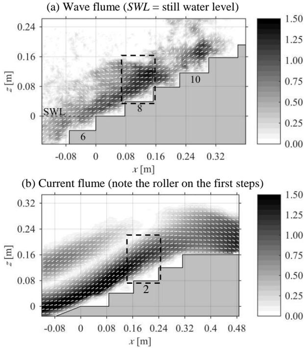
**Figure 9.** Velocity fields in [m/s] for the full fields of view and both setups (only every 5<sup>th</sup> vector is displayed; vector lengths are normalized for better legibility).
