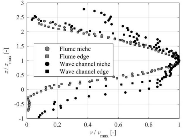
**Figure 11.** Normalized velocity distributions at upstream step edges and over the step niche ( $z = 0$  at the pseudo-bottom), step 8 for the wave channel and step 2 for the current flume (see Figure 9).
