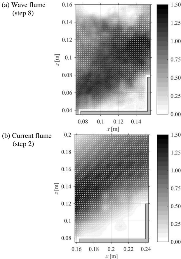
**Figure 10.** Velocity fields in [m/s] for selected steps and both setups (only every 5<sup>th</sup> vector is displayed; vector lengths are normalized for better legibility).
