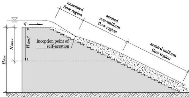
**Figure 5. Flow regions in skimming flow regime on stepped spillways (identical to smooth spillway flows)**
