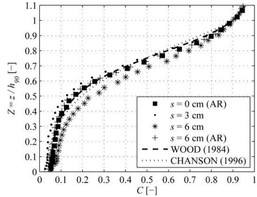
**Figure 9. Air concentration distributions in uniform flow region ( $\varphi = 26.6^\circ$ ,  $q = 0.11 \text{ m}^2/\text{s}$ , AR: artificial roughness, data at step edges for stepped spillway models) in comparison to theoretical models by [3] and [7] with  $\bar{C} = 0.30$**
