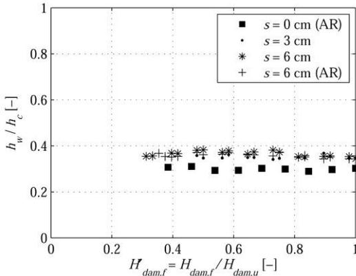
**Figure 7. Development of clear water depth  $h_w$  in non-uniform flow region ( $\varphi = 26.6^\circ$ ,  $q = 0.11 \text{ m}^2/\text{s}$ , AR: artificial roughness)**
