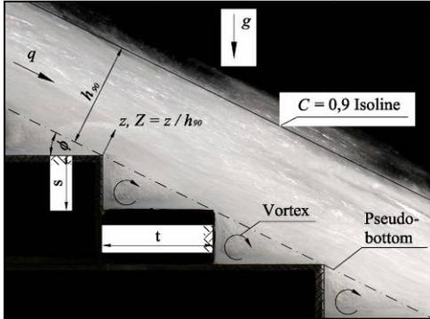
**Figure 2. Sketch of skimming flow on an embankment stepped spillway compared to physical model test ( $\varphi = 26.6^\circ$ ,  $s = 6$  cm,  $q = 0.11$  m<sup>2</sup>/s)**
