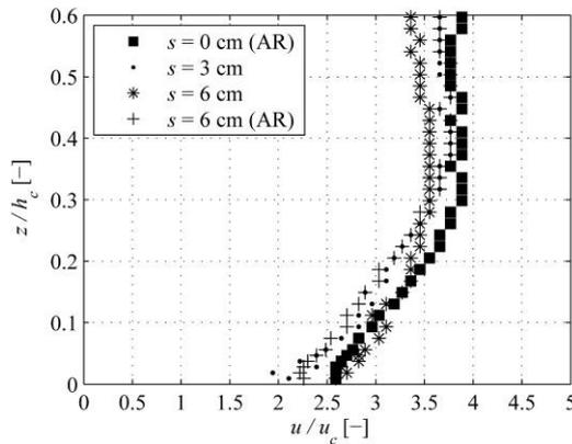
**Figure 10. Velocity distributions in uniform flow region ( $\phi = 26.6^\circ$ ,  $q = 0.11 \text{ m}^2/\text{s}$ , AR: artificial roughness, data at step edges for stepped spillway models)**
