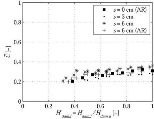
**Figure 8. Development of mean air content  $\bar{C}$  in non-uniform flow region ( $\varphi = 26.6^\circ$ ,  $q = 0.11 \text{ m}^2/\text{s}$ , AR: artificial roughness)**
