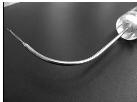
**Figure 4. Double-tip conductivity probe for measuring of air content and flow velocities (note: 2 electrodes with a distance in flow direction of 5.1 mm)**
