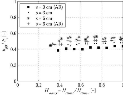
**Figure 6. Development of air-water mixture depth  $h_{90}$  in non-uniform flow region ( $\varphi = 26.6^\circ$ ,  $q = 0.11 \text{ m}^2/\text{s}$ , AR: artificial roughness)**
