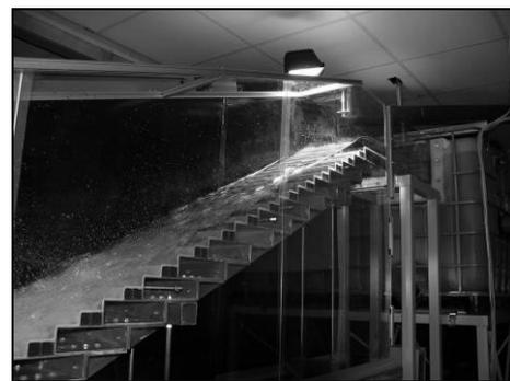
**Figure 1. Physical model with  $H = 2.34$  m,  $\phi = 26.6^\circ$ , step height  $s = 3$  cm and specific discharge  $q = 0.09$  m<sup>2</sup>/s (note the clear water region near the spillway crest)**
