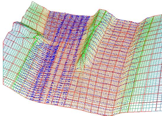
Figure 2: Measurement points, de Boor point grid and b-spline surface
