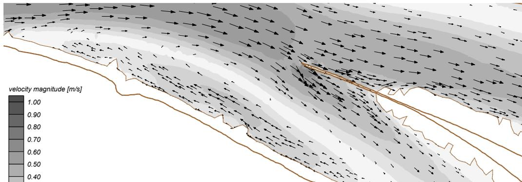
Figure 7: Model results for M1 ( $Q=150\text{m}^3/\text{s}$  at gauge Intschede,  $TS=14.5$ )
