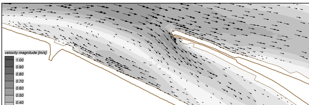
Figure 8: Model results for M3 ( $Q=150\text{m}^3/\text{s}$  at gauge Intschede,  $TS=14.5$ )
