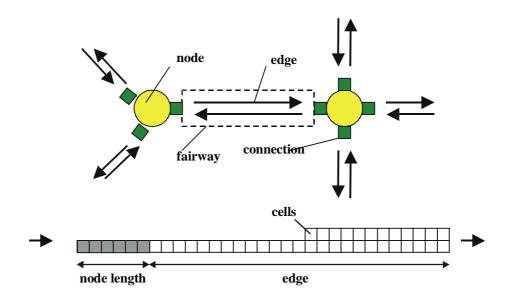
Fig. 3: Network Design with Edges/Nodes and Edge Splitting to model Vessel Traffic on Inland Waterways
