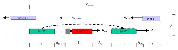
Fig. 4: Parameters used for Passing Simulation in WABIS Traffic Simulation Module
