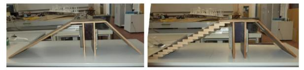
Fig. 2. A view of the submerged breakwater model set-up with smooth and stepped front slope
