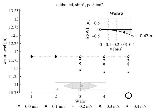
**Figure 7. Water levels in outer harbor and lock chamber for different ship velocities (ship 1, position 2, outbound)**
