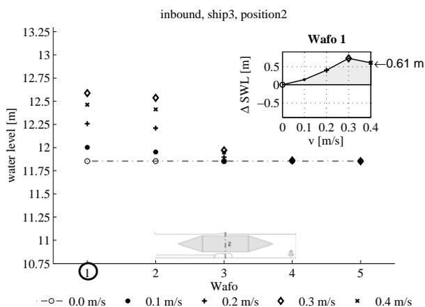
**Figure 5. Water levels in outer harbor and lock chamber for different ship velocities (ship 3, position 2, inbound)**
