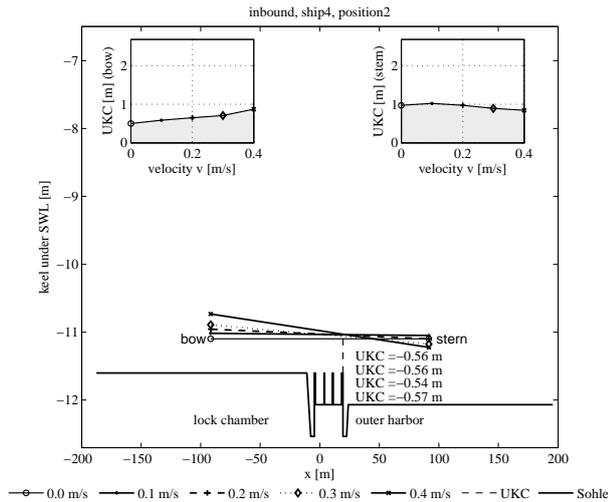
**Figure 8. Keel position during inbound process of ship 4, position 2 with remaining UKC for different ship velocities**
