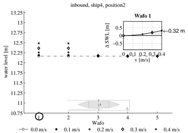
**Figure 6. Water levels in outer harbor and lock chamber for different ship velocities (ship 4, position 2, inbound)**
