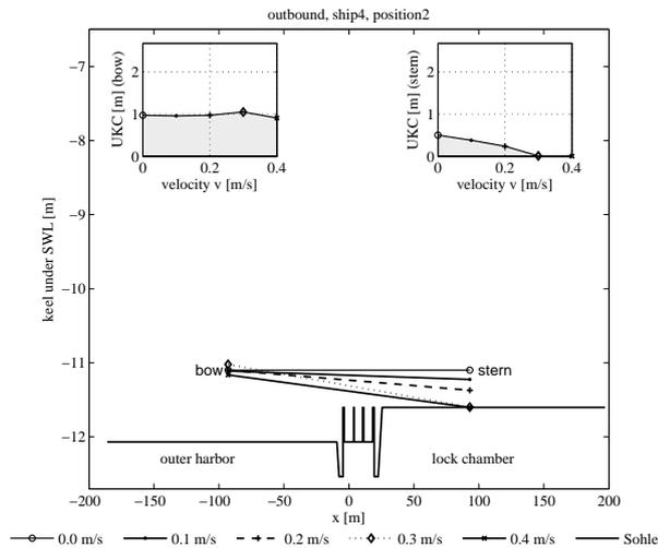
**Figure 9. Keel position during outbound process of ship 4, position 2 with remaining UKC for different ship velocities**
