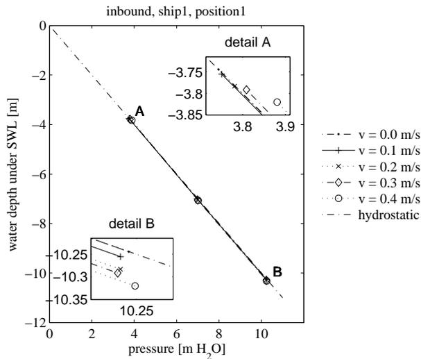
**Figure 11. Vertical pressure distributions between ship hull and lock gate (inbound, ship 1, position 1)**
