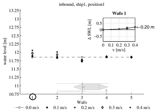
**Figure 2. Water levels in outer harbor and lock chamber for different ship velocities (ship 1, position 1, inbound)**
