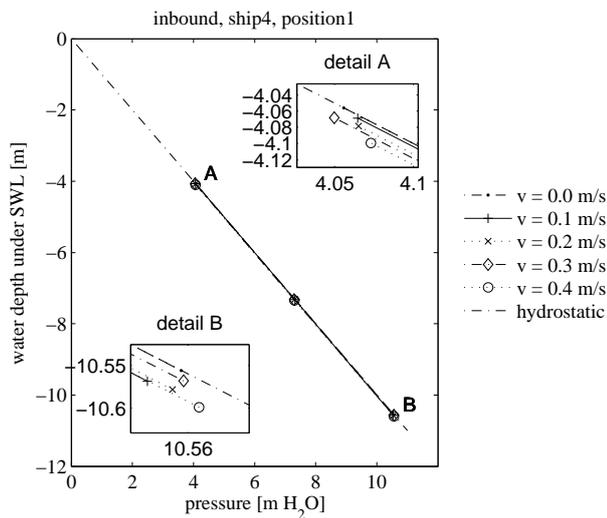
**Figure 12. Vertical pressure distributions between ship hull and lock gate (inbound, ship 4, position 1)**
