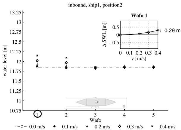
**Figure 3. Water levels in outer harbor and lock chamber for different ship velocities (ship 1, position 2, inbound)**
