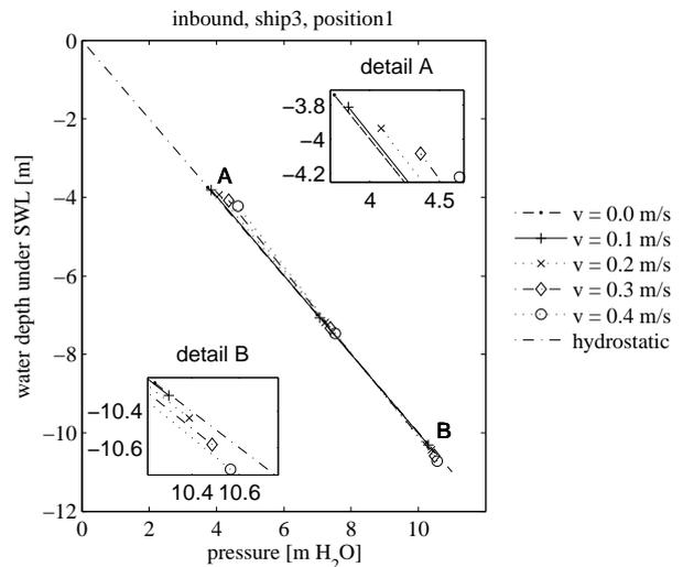
**Figure 10. Vertical pressure distributions between ship hull and lock gate (inbound, ship 3, position 1)**
