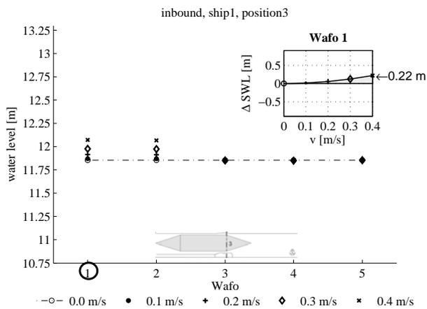
**Figure 4. Water levels in outer harbor and lock chamber for different ship velocities (ship 1, position 3, inbound)**
