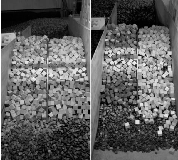
Figure 3: Armor layer before (left picture) and after (right picture) loading with regular waves (left side of armor layer: heavy concrete cubes, right side of armor layer: normal concrete cubes)
