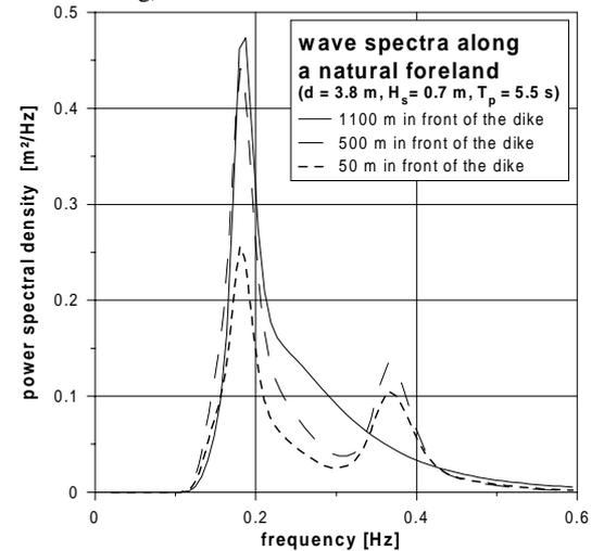
Fig. 9: Wave Spectra along a Natural Foreland for a Water Depth of 3.8 m, a Significant Wave Height of 0.7 m and a Peak Period of 5.5 s at different Positions in front of the Dike (Results of Numerical Modelling)
