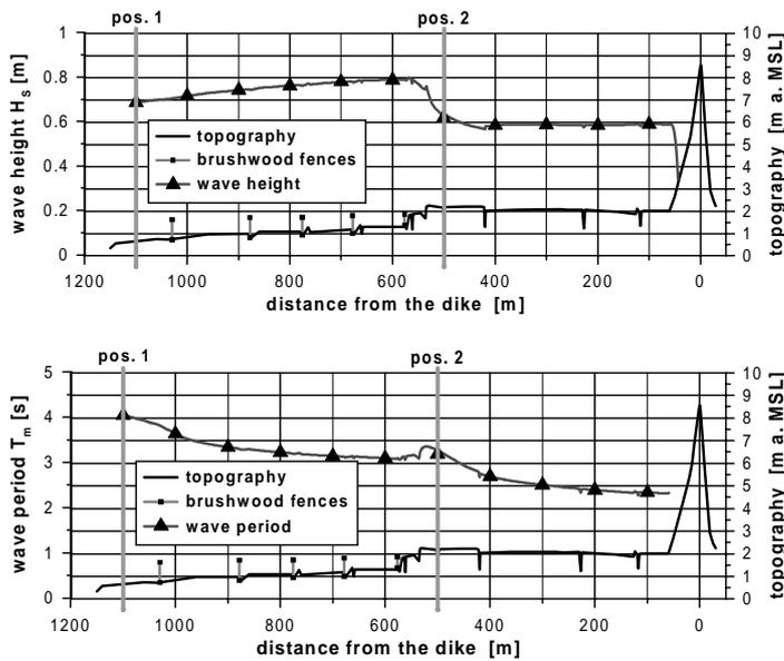
Fig. 4: Wave Parameter over a Foreland at the Coast of Dithmarschen – Significant Wave Height (top) and Mean Wave Period (bottom) for a Water Level of 3.8 m a. MSL and a Wind of 20 m/s and 300° (Mai and von Lieberman, 2001)
