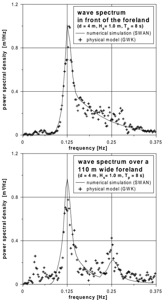
Fig. 7: Wave Spectrum in front of the Foreland (left) and over a 110 m width Foreland (right) for a water depth of 4 m, a Significant Wave Height of 1 m and a Peak Period of 8 s (Results of Physical and Numerical Modelling)
