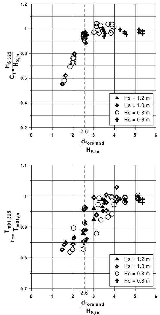
Fig. 6: Effects of a 1.4 m high Foreland on Wave Height (left) and Effects on Wave Period (right) 325 m behind Seaward Drop carried out with the Model SWAN (von Lieberman and Mai, 2000b)
