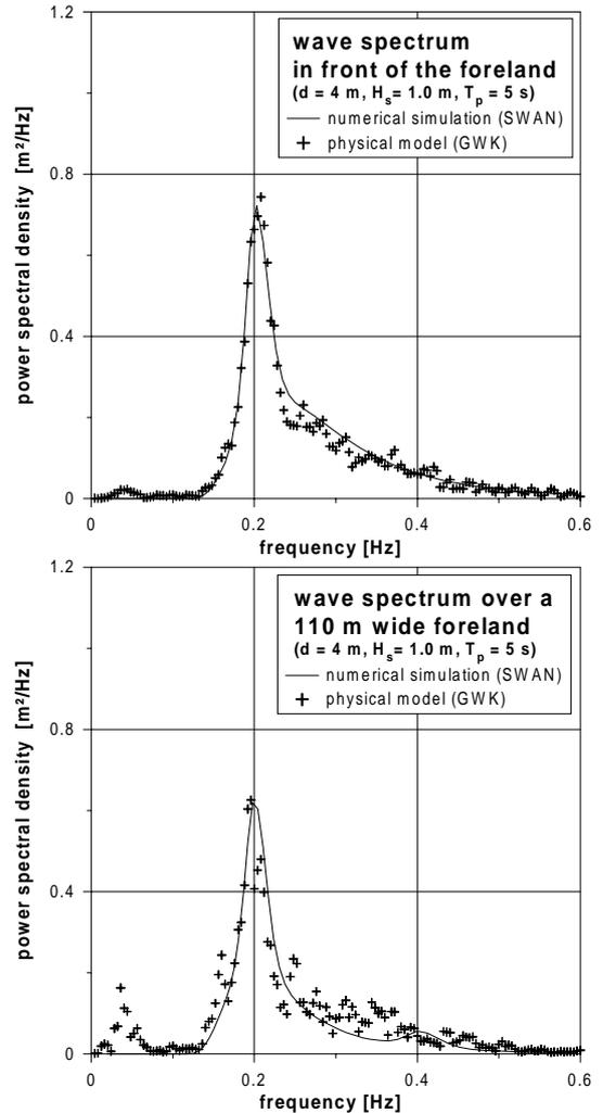
Fig. 8: Wave Spectrum in front of the Foreland (left) and over a 110 m width Foreland (right) for a Water Depth of 4 m, a Significant Wave Height of 1 m and a Peak Period of 5 s (Results of Physical and Numerical Modelling)
