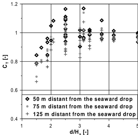
Fig. 5: Transmission Coefficient  $c_T$  as a Function of Relative Water Depth over the Foreland within the Large Wave Tank at different Distances from the Seaward Drop (Mai und von Lieberman, 2001)
