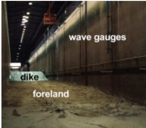
Figure 2: Experimental set-up in the GWK
