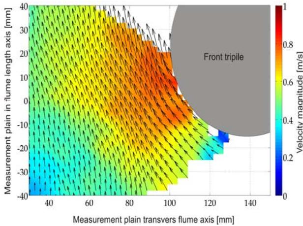
Figure 3. Vector field of horizontal velocities near the front tripile for extreme wave conditions, upper measurement plain during wave crest propagation along the tripile
