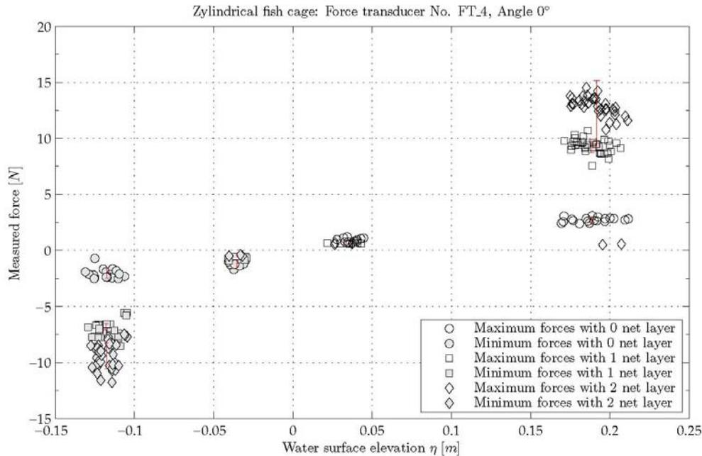
Figure 6. Correlation of maximum wave heights and measured forces for cylindrical fish cages for force transducer FT\_4 with respect to the number of net layers
