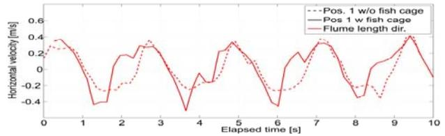
Figure 4. Horizontal velocity from PIV-measurements comparing setup with and without fish cages assembled
