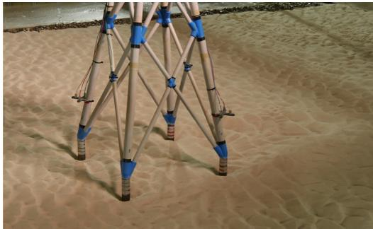
Abb. 3. Exemplary photo of the model setup and scour pattern
