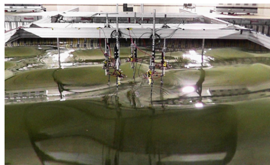
Abb. 2: Bichromatic-Bidirectional waves tested at the 3D wave basin in Marienwerder
