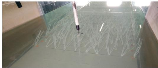
Abb. 1: Artificial seagrass meadows in the circular track-flume. ADV probe used to measure and develop velocity profiles before, within and after the meadows.
