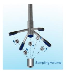
The Vectrino velocimeter operating principle: A pulse is transmitted from the centre transducer, and the Doppler shift introduced by the reflections from particles suspended in the water, is picked up by the four receivers.
