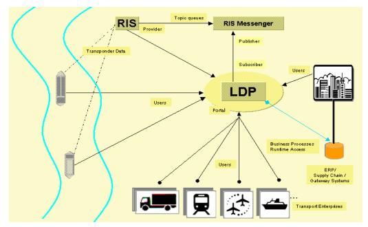
Figure 2-1: RIS/LDP Connectivity for registered Users through a common Interface (Portal)
