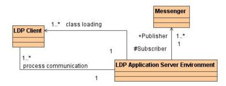
Figure 3-5: Asynch 2-way C/S Communication
