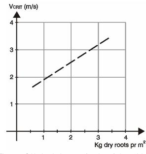
Fig. 7: Critical velocity as a function of dry weight of grass roots in turf.
